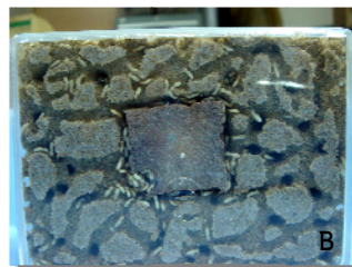
Figure 2.Laboratory test (A) In plastic block (B)Termites attackedwood
